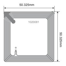
**Antenna Design** Top: Aluminum 30 µm Substrate: PET 38 µm Bottom: Aluminum 10 µm
