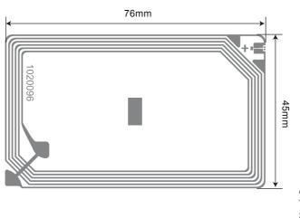
Antenna Design Top: Aluminum 30 μm Substrate: PET 38 μm Bottom: Aluminum 10 μm
