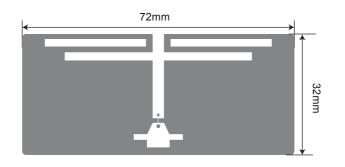
Antenna Design Top: Aluminum 10 μm Substrate: PET 50 μm/Paper 60 μm
